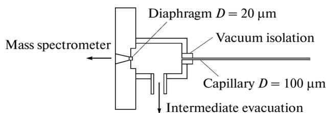
Fig. 1. Unit for the delivery of a sample into the mass spectrometer.
