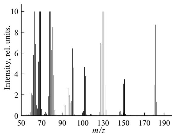
Fig. 2. Mass spectrum of a gaseous mixture in an IAM circuit in the range of  $m/z$  55–200. Peaks with  $m/z$  69, 131, 181, and 199 correspond to ions produced by the electron ionization of sevoflurane.
