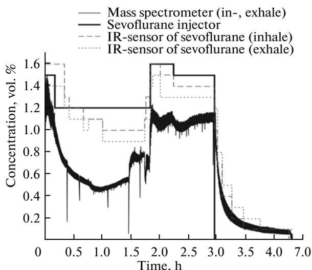
**Fig. 5.** Time dependence of sevoflurane concentration according to the readings of the injector, mass spectrometer, and IR-sensor (for Dragger Julian IAM).
