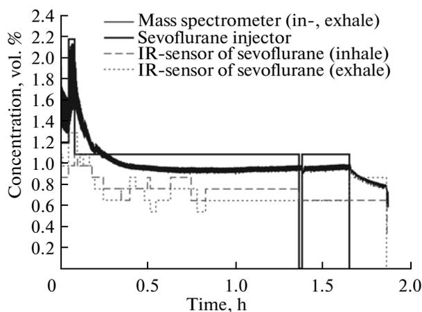
**Fig. 4.** Time dependence of sevoflurane concentration according to the readings of the injector, mass spectrometer, and IR-sensor (for Dragger Julian IAM).
