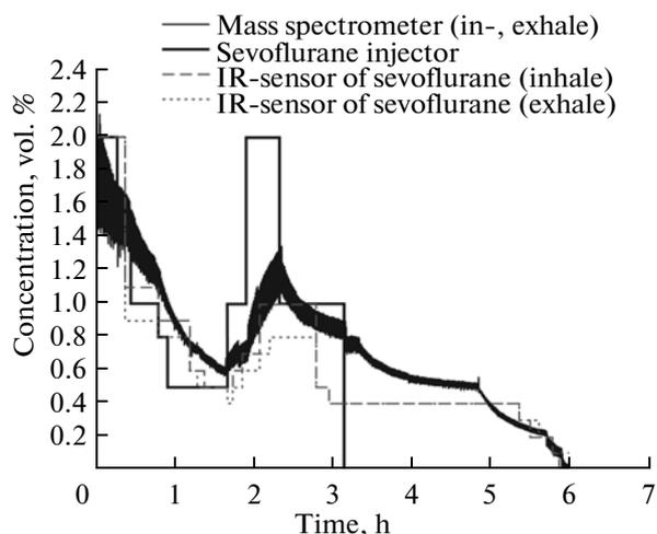
**Fig. 3.** Time dependence of sevoflurane concentration according to the readings of the injector, mass spectrometer, and IR-sensor (for Dragger Julian IAM).
