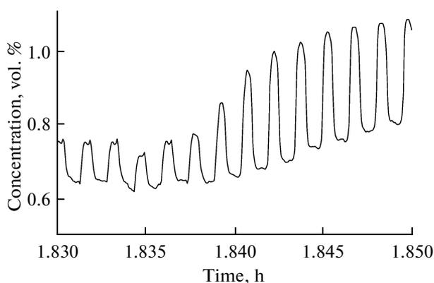
**Fig. 7.** Dynamics of concentration evolution for sevoflurane in an increase in the anesthetic concentration in the IAM circuit over a breathing cycle.
